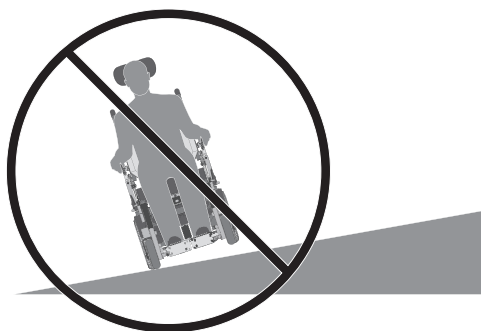
Figure 4. Do not turn on a slope.
