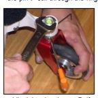
the hole of the ring **A1** to control its position and, with the other bare hand, screw up the nut **B** as much as possible while checking the spirit level. Now gradually tighten the nut **B** with the 18 mm spanner. If, while tightening, the bubble moves away from the circle, it means that the fork has moved. To compensate such unwanted movement, turn the fork in the nut loosening direction and check the bubble. It may seldom happen, though, that even the ring **A1** moves
