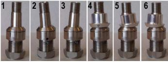
Pictures 1, 2 and 3 show that the upper axle of the bearing unit, rotating on the lower axle (that allows the fork to turn), changes inclination thanks to the inclined plane of the ring **A2**. Pictures 4, 5 and 6 show three different inclinations of the ring **A1** keeping **A2** still. Each combination of the position of these two rings gives a different angle to the fork axis.
