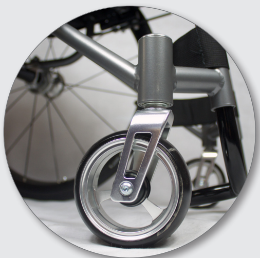
Aluminium castor housing cap and low ride castor forks
