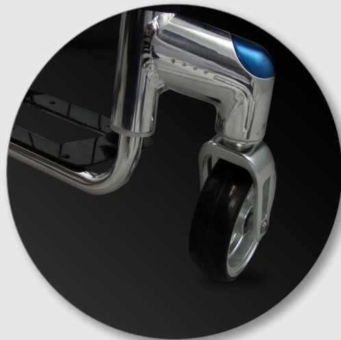
Super light castors, 4" x 1.25" with aluminium centre
