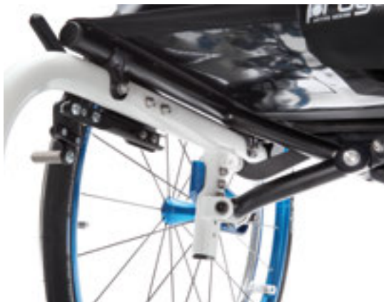
Rear axis crossbar hidden under the seat.
