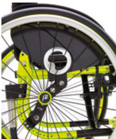
Dynamic rear frame with multi-adjustment rear wheel jointed plate, backrest angle adjustment and mudguard with rotative adjustment system.
