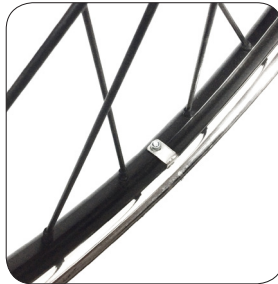
XL090 - Handrim remove excess mounting tab
